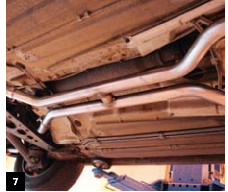
7 Where once there was a centre silencer, now there are straight-through pipes
