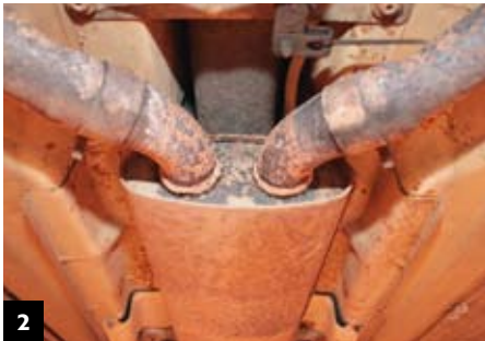
2 This is the standard centre silencer box. Our Milltek Super Sport replacement system would do away with this in favour of straight-through pipes
