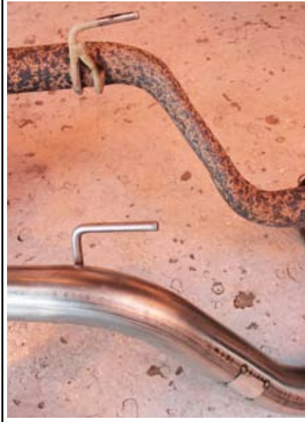
5 The replacement system laid bare in the floor – note the straight through pipes in lieu of the centre silencer. The inset shows how the over axle pipes are constant radius – the standard ones are 'pancaked'
