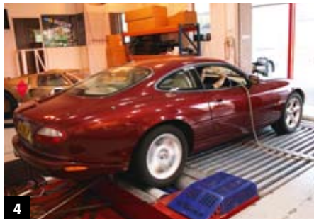
4 With the remap downloaded and the car having been left to idle for five minutes, it's taken through several full power runs through the gears to check all is well
