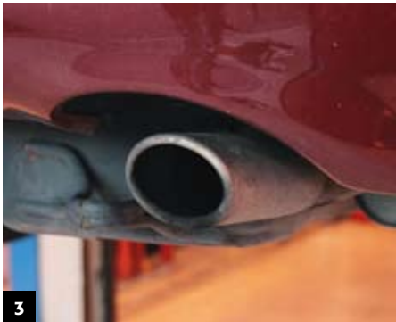
3 After the centre silencer, the standard system branches into two separate pipes again which run up and over the axle to end in these rather weedy looking tailpipes
