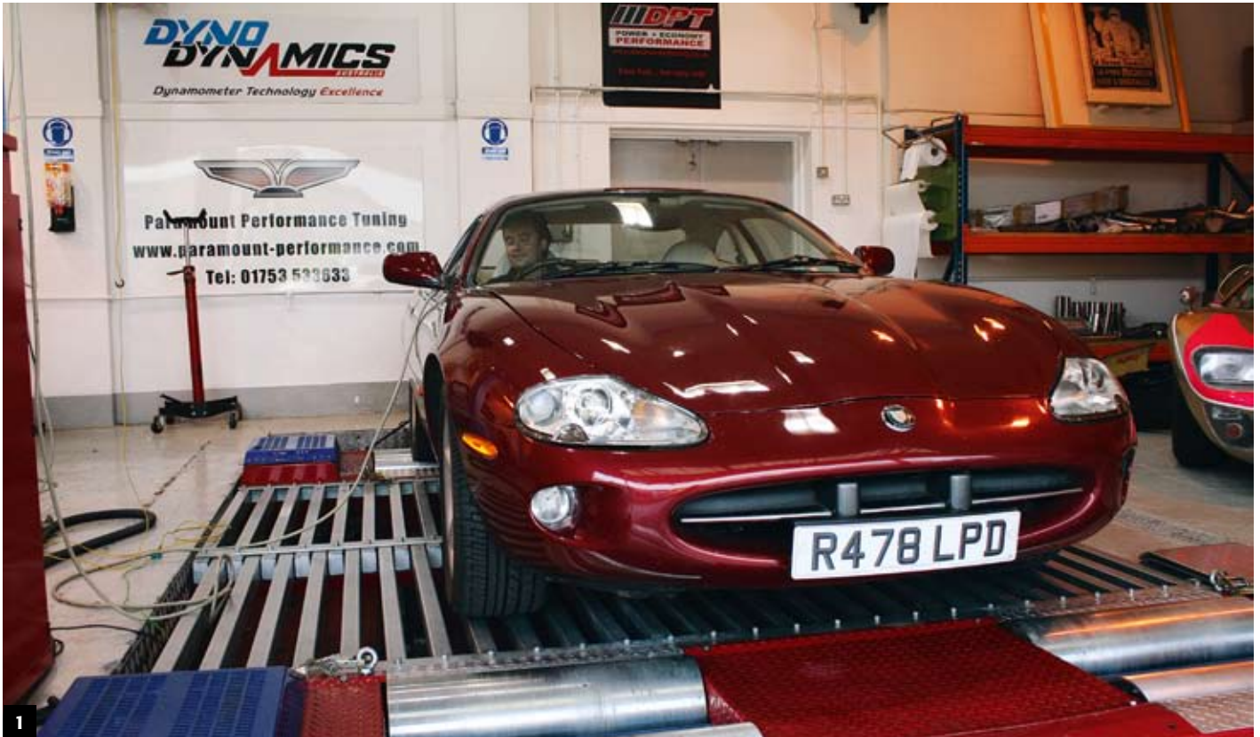
1 Paramount's rolling road is a serious piece of kit... Here, our car is put through its paces to ensure the engine is healthy before the remap begins
